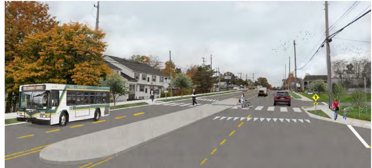
FIGURE 13 Proposed mid-block crossing with pedestrian island
