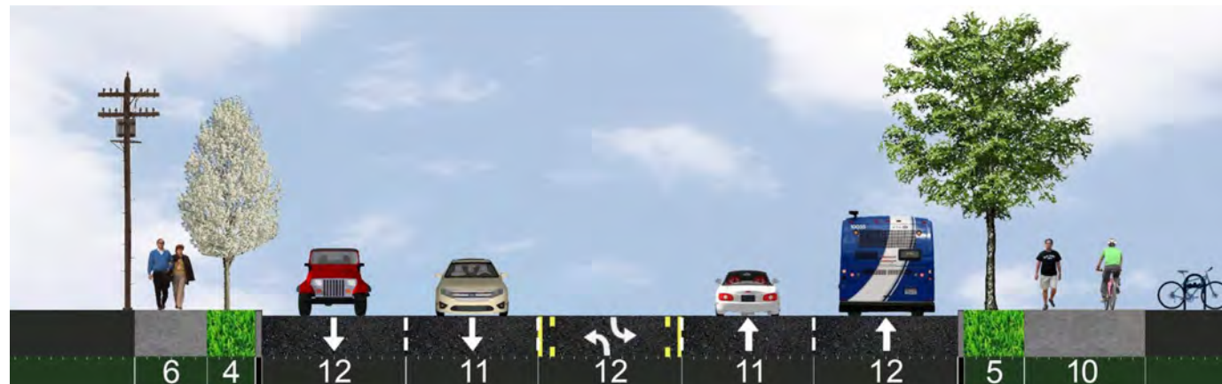
FIGURE 3 Proposed corridor right-of-way and lane widths
