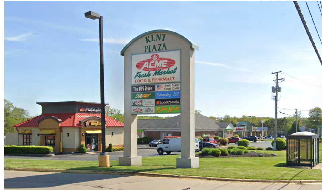
FIGURE 11 Bus shelter near Pizza Hut is accessible from the road/bus but there is no pedestrian access from the bus stop to the business entrance. A person in a wheelchair would be forced to navigate around the lawn by using the driveway, which would put them at risk.
